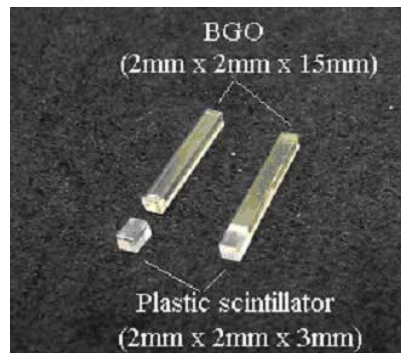
Fig. 4 Photograph of phoswich scintillator, before optical coupling (left) and after optical coupling (right).
